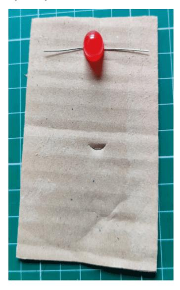
3. Take a bit of copper tape or glue and some aluminium foil over the long leg of the red LED.
